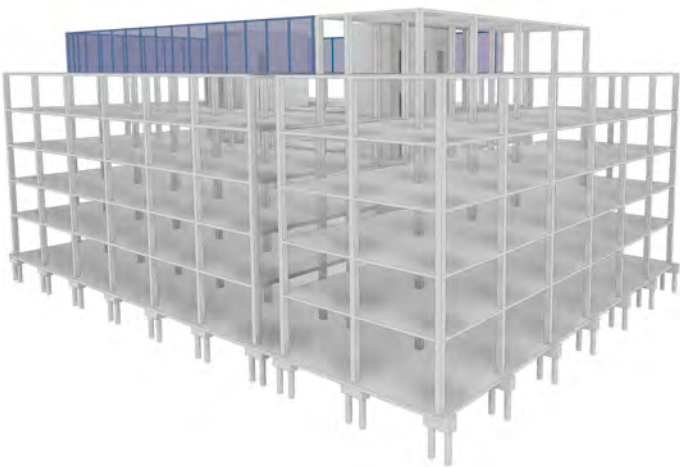
Baseline RC frame for labs and offices
